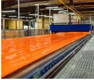
The Omega UV Liner is constructed with ECR (corrosion-resistant) fiberglass and advanced UV resins – proven to be one of the strongest on the market. Omega Liners are manufactured using unsaturated polyester or vinyl ester resins for environmentally conscious projects and are offered from 6" (150mm) to 66" (1675mm).
