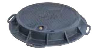
Trumbull Manufacturing composite manhole frames and covers offer superior corrosion resistance to H2S gas and are lighter weight compared to cast iron. Other benefits include AASHTO H20 & H25 traffic rating and O-ring sealed for water infiltration. Trumbull also offers wall sleeves and Link-Seal® for creating and sealing wall penetrations in concrete vaults and other underground boxes.
