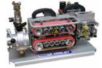
The Plumett MiniJet™ is highly effective, and significantly increases daily production. The belt-drive system ensures excellent cable grip without damage, and the clamping system absorbs cable diameter tolerances. In addition, its advanced design and construction improve installation performance. Its components are selected and manufactured to meet the highest requirements.
