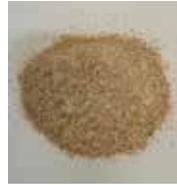
Eco-Solidify is a liquid and sludge solidification agent that blends wood sawdust and super absorbent polymer in
