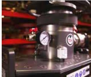
With its revolutionary connection design, the POLYSTOPP® Quick Connect system makes it easy to safely perform hot tapping, plugging and branching on polyethylene (PE) pipelines – and do it faster than with any other isolation technology. The system is lightweight and simple and uses significantly less excavation space.
