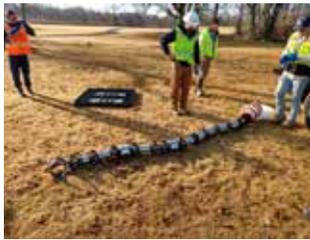
RFT tools are used to inspect metallic pipes by using high-resolution electromagnetic technology to create an energy field that passes through the pipe to measure the thickness of the pipe wall. The information is then used to create a detailed mapping of the cylinder.
