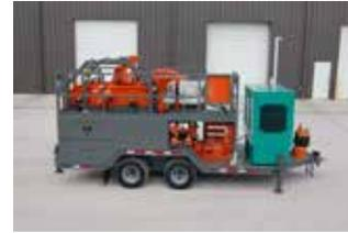
Tulsa Rig Iron's MCS-330 mud reclaimer is a great pairing for 40K to 60K drills. Featuring a normal cleaning volume of 240 GPM, 2200-gallon tanks, rear discharge shaker, and built as a robust integrated trailer design, this model is a true workhorse.
