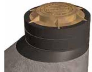
WrapidSeal™ manhole encapsulation system consists of an engineered primer and a unique, wrap-around, heat-shrinkable sleeve designed specifically to seal joints and prevent groundwater from entering a collection system. WrapidSeal™ can be utilized on both new construction and rehabilitation of existing manholes.
