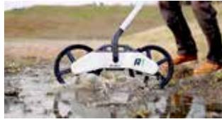
The TeraTrak R1 is a topo mapping tool that produces full, achievable bore plans that help drillers work faster and safer. How? By taking hyper-accurate topography readings and combining them with infrastructure locations and waypoints, the R1's algorithm produces a rod-by-rod plan. Simply put, it does the math for drillers.
