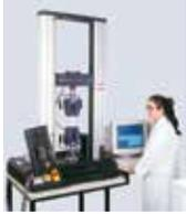
HTS Pipe Consultants is a materials-testing and consulting firm specializing in cured-in-place vinyl ester, polyester, epoxy and glass fiber-reinforced resins. Services include the determination of flexural and tensile strength, flexural creep and chemical-resistance properties. All testing is performed in accordance with ASTM, Greenbook and ISO standards.
