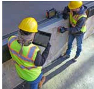
Meet Flex NX®, the industry's most powerful and efficient concrete scanner. The two data collection modes will lead to streamlined testing for structural safety and simplify concrete scanning. Two wireless antennas offer greater flexibility for challenging job sites, as well as a host of other technological advancements that redefine the scanning workflow.
